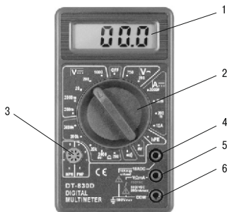
Figure 1 – Multimeters front panel elements
